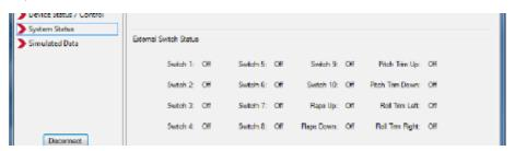
Turn a switch on and verify that the corresponding switch input changes from OFF to ON. Then turn it off and go to the next switch input. Be sure to verify that the trim and flap switches are wired in the correct direction. It is easy to get these backwards. If you turn a switch on and it does not change the status display, or changes the wrong display, then the switch is wired incorrectly.
