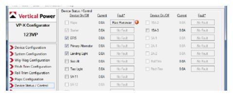
Check that there are no faults on a device. If there is a fault, note the TYPE of fault. That can help you understand the cause of the fault. Faults are explained in the VP- X Installation Manual. You can reset a fault by pressing the button that describes the fault.
