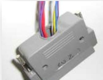
Wires can vibrate within the connector housing
