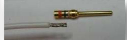
Step 3: Install terminal into crimper tool, ensuring crimp tool is adjusted to the proper height. The head of the terminal should be flush with the top of the tool.
