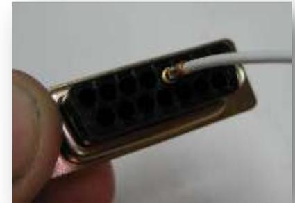
Step 5: Insert terminal into connector assembly until you hear a slight click. Give the wire a tug to make sure it is fully seated. Visually inspect the other face of the connector to verify proper placement of the terminal.
