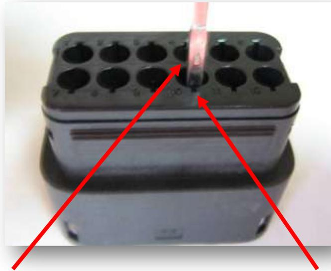
**Orientation feature aligned with index**
