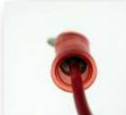
Wires can vibrate near the connector
